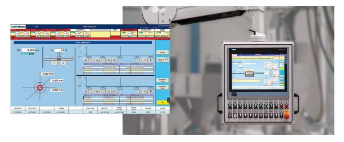
The Bellaform operating interface outputs process data such as temperature curves of the extruder heating or pressure curves in the vacuum tank as a trend curve in real time. Diameter and wall thickness, the distance between the nozzle exit and the calibration or the temperatures in the vacuum tank are recorded. All relevant data are provided in a format that permits further processing or archiving in a superordinate central control.
