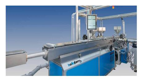
Bellaform offers two vacuum tanks for different product diameters each (25–50 mm). Both versions can be combined easily with any of our extrusion lines.
